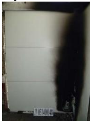
Fig. 3 After SBI Test
