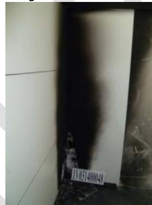
Fig. 4 After SBI Test
